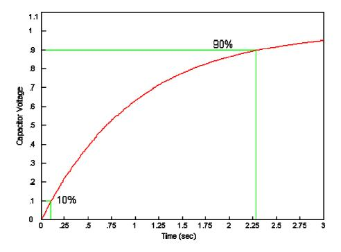
In case of the RC network, the 10% level is reached after 0.105 time constants and the 90% after 2.302 time constants; thus the rise time is (2.302 - 0.105) time constants which is 2.197 time constants or  $2.197\tau$ . We'll call it  $2.2\tau$  for simplicity.
