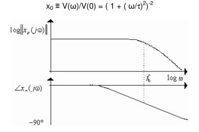
Using the dB logarithmic scale where the attenuation X<sub>0</sub> is expressed in dB as
