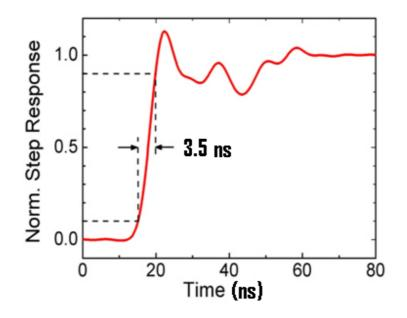
A 'scope whose bandwidth is 100 MHz and whose step response is that of a simple RC network will have an internal rise time of 3.5 ns. Therefore, a pulse with rise time shorter than this cannot be measured on such a 'scope and it is fruitless to attempt to measure the rise time of a pulse if it is shorter than that of the 'scope's. Even signals whose rise time approaches that of the 'scope will be distorted so that their measured rise time is increased. The measured rise time is given by:
