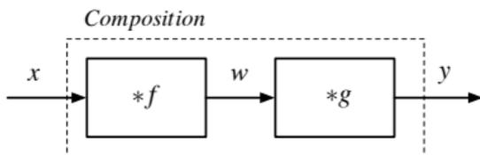
is the same as a single system with an impulse response  $h = f * g$
