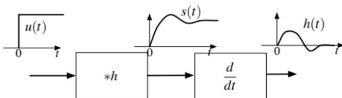
To show this, commute the convolution system and the differentiator to produce a system with the same overall impulse response
