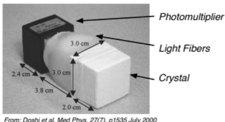
These are used in Positron Emission Tomography (PET) systems. Input is a sequence of impulses (photons).
