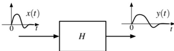
If  $H$  is a linear system, its zero-input response is zero. Homogeneity states if  $y = F(ax)$ , then  $y = aF(x)$ . If  $a = 0$  then a zero input requires a zero output.
