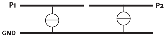
Figure 10: Test board configuration for adjacent power nets
